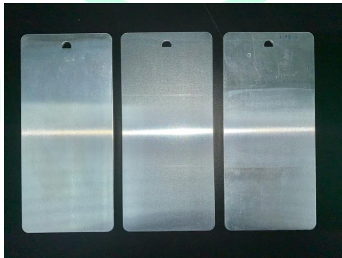
Visual appearance of plate after scrub resistance test. L: Freshly mixed product; M: After 2 months at 50 °C; R: Example of plate with film loss.
